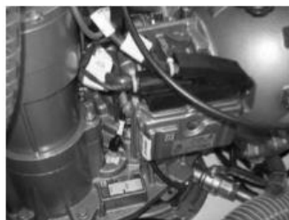
Boîtier TCU (Transmission and Clutch Management) (Repère 5)
